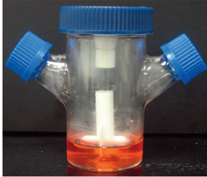
FIGURE 5.16 A spinner flask, commonly used for tissue engineering applications. Photo courtesy of Prof. Taby Ahsan, Tulane University.
